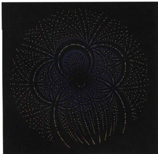
Fig. 19. Simulation of Laue diffraction pattern corresponding to Fig. 18(a). The colours of the diffraction spots represent the different wavelengths present, between 0.25 Å (blue), through the colours of the rainbow, and 1.5 Å (red). For multiple spots the longest wavelength present is shown.
