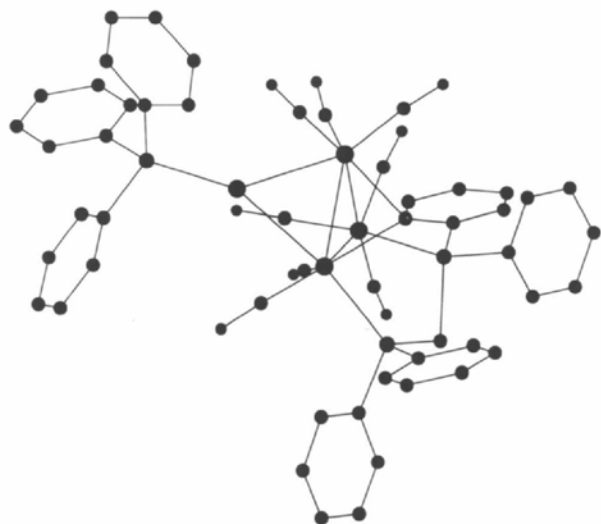
Fig. 22. The structure of the organometallic cation \text{AuOs}_3\text{H}(\text{CO})_8[\text{Ph}_2\text{PCH}_2\text{P}(\text{Ph})\text{C}_6\text{H}_4](\text{PPh}_3) established entirely from Laue diffraction photographs of a small crystal of its hexafluorophosphate. Space group C2/c . The large circles represent Au or Os atoms; the others in order of decreasing size are P, C and O.
